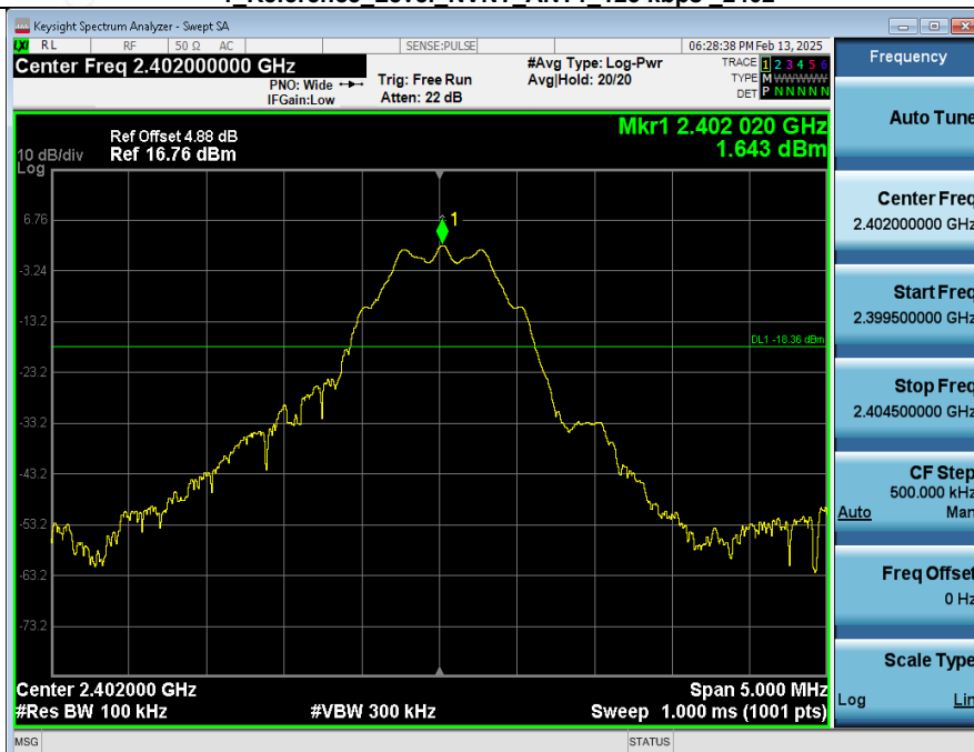
2 Spurious Emission_NVNT_ANT1_125 kbps_2402
