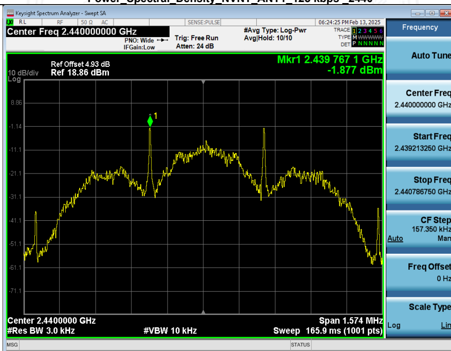
Power Spectral Density NVNT ANT1 125 kbps 2440
