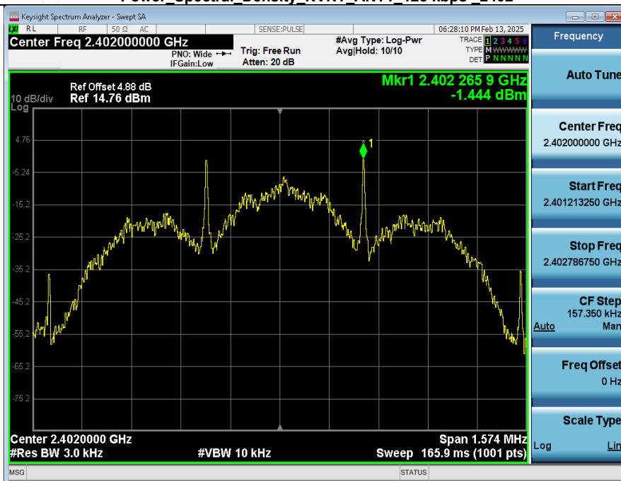
Power Spectral Density NVNT ANT1 125 kbps 2402
