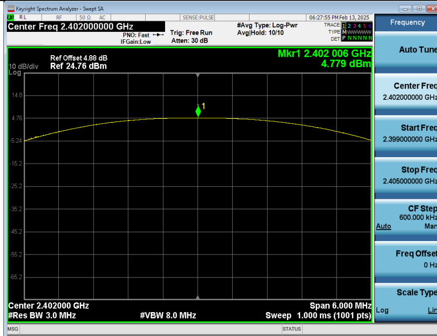
Peak Output Power NVNT_ANT1_125 kbps_2402
