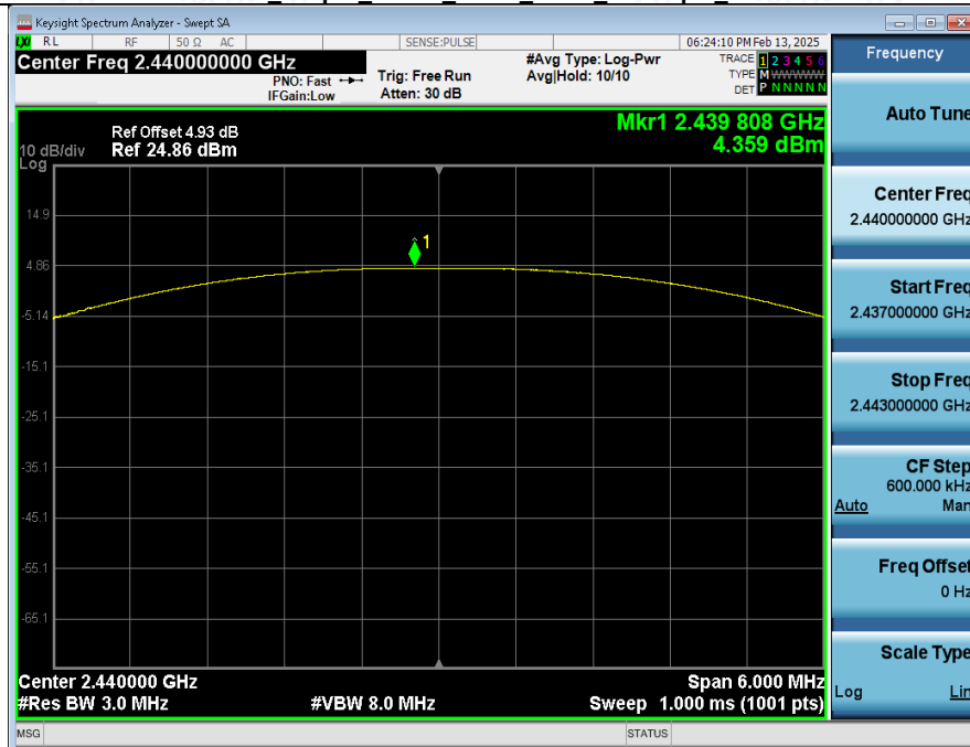
Peak Output Power NVNT_ANT1_125 kbps_2440
