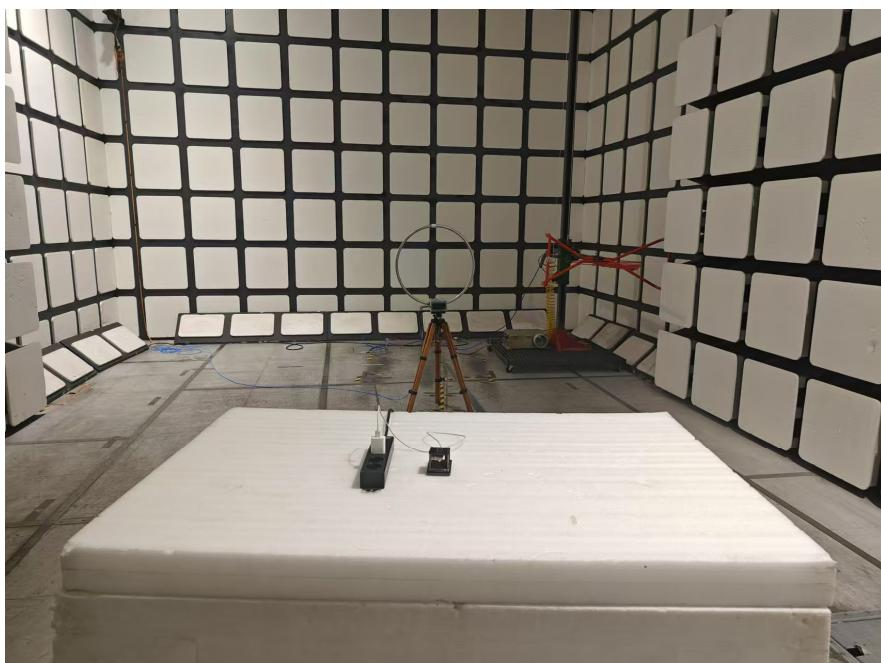
**Radiated Emissions View (Below 30MHz) - Ground-parallel**
