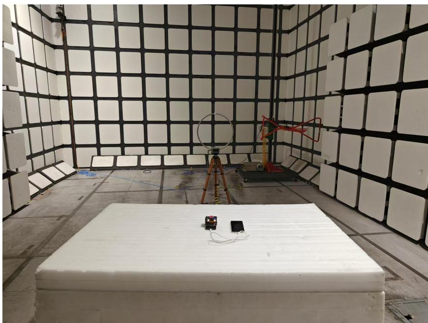
**Radiated Emissions View (Below 30MHz) - Ground-parallel**
