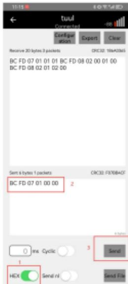
**Step2:** In the startup state, after the APP sends a test request to the device, the TB-01 will enter the
