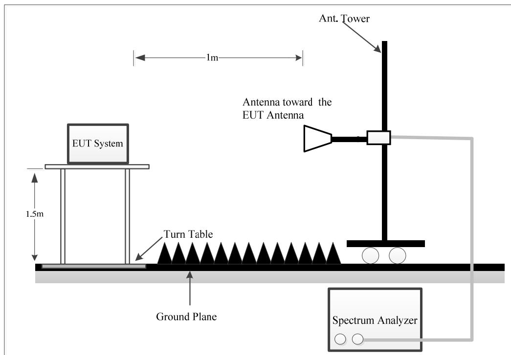
Place the measurement antenna at a measurement distance that is in the far-field of the measurement antenna, in the far-field of the EUT antenna. The EIRP test was performed at 1m distance, which was larger than the minimum test distance, please refer to section 4.4.4 for more detail.
