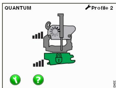
LockSense can be present on both machine worktool attachments and tiltrotator attachments. The illustration on the left is an example of a complete combination when both attachments are installed.
