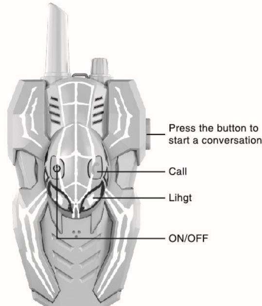
After power on, press talk button to speak and send voice, release to receive. Double-click the talk button of device A, and device B will ring a call tone.
