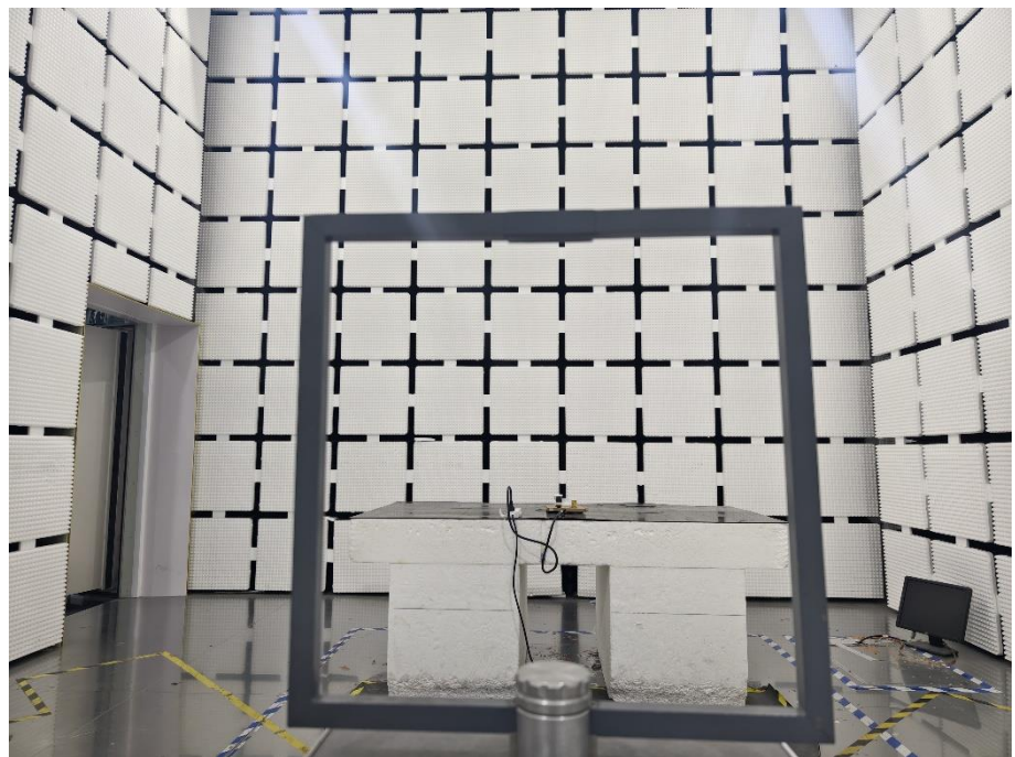
Radiation Emission Test Setup (Below 30MHz)
