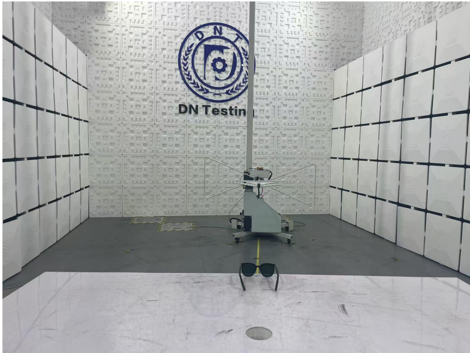
Radiated Emission Test View|(Below 1G)
