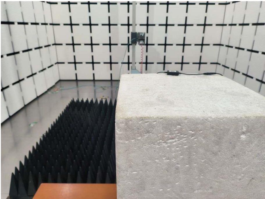
Radiated Emission Test View Above 1GHz
