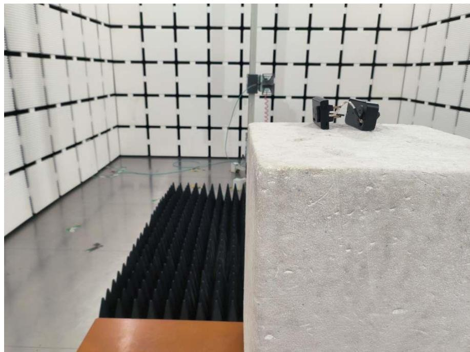
**Radiated Emission Test View Below 30MHz**
