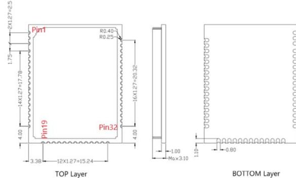
Figure 2 Dimensional drawing (unit mm)
