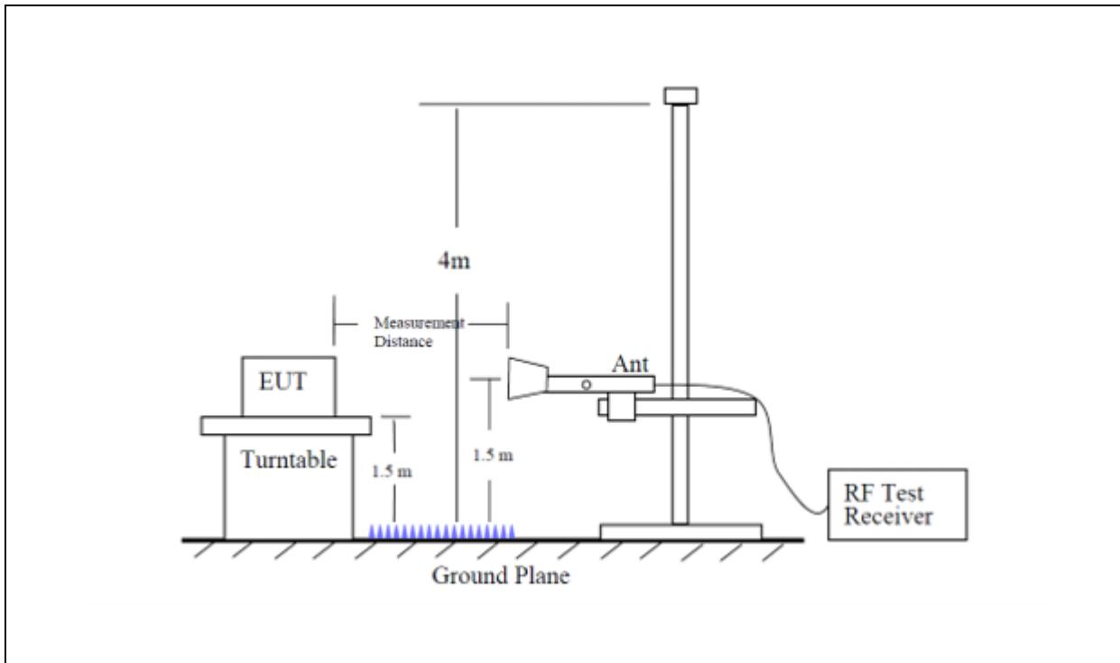
**TEST SITE DIAGRAM – ABOVE 18 GHz**
