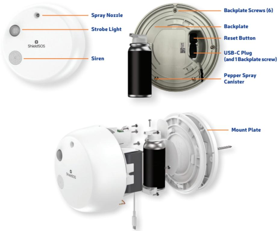
**Warning:** Do not use power tools, hand tighten red screws only.
