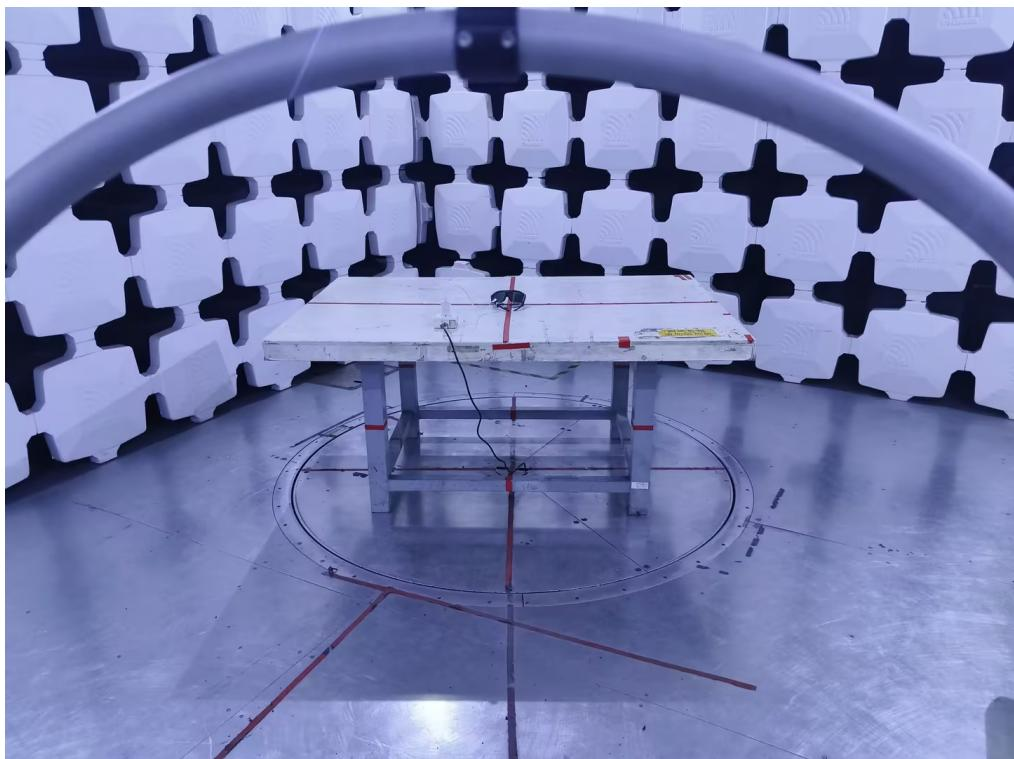
**Radiated Emissions Test Photos****30 MHz to 1000 MHz**
