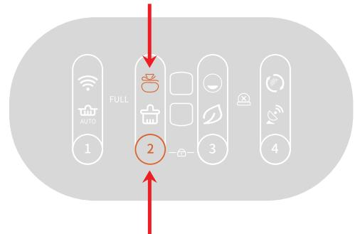
Long press for 2 seconds to start the waste bag change mode immediately.
