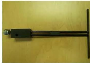
Figure 1 – MVG COMOSAR Validation Dipole
