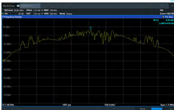
8DPSK on Channel 78
