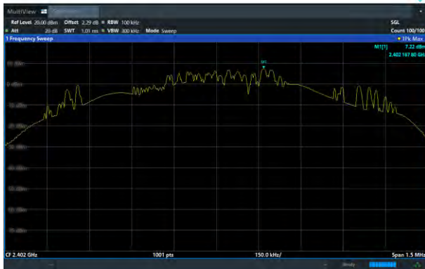
8DPSK on Channel 00
