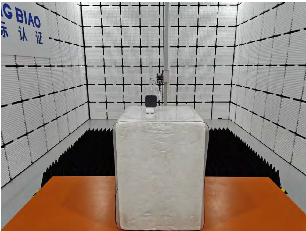
Radiated Emission Above 1GHz
