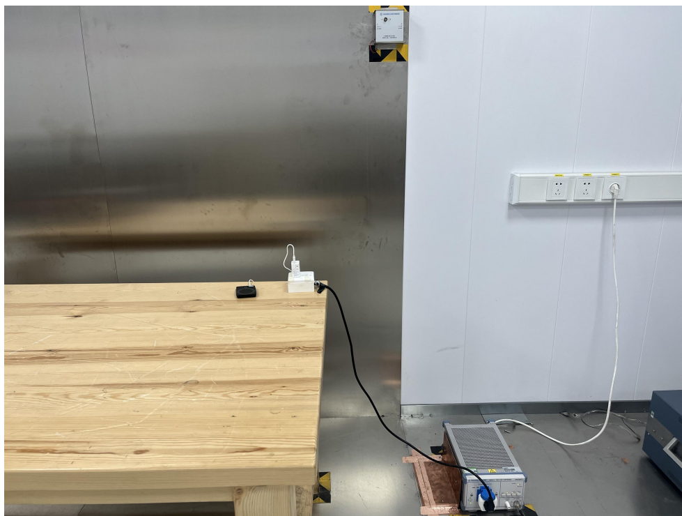
Radiated Emission Test View|(Below 1G)
