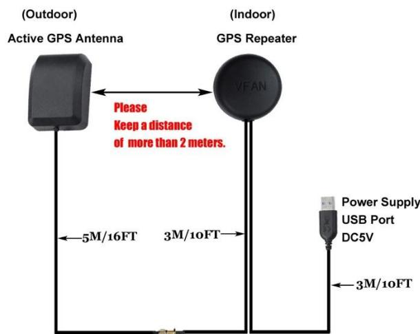
VFAN GPS Signal Booster Amplifier Signal Strength Active Antenna for Car/Trucks/Indoor Use, Gain 30 dB, with Magnetic Base and Waterproof
