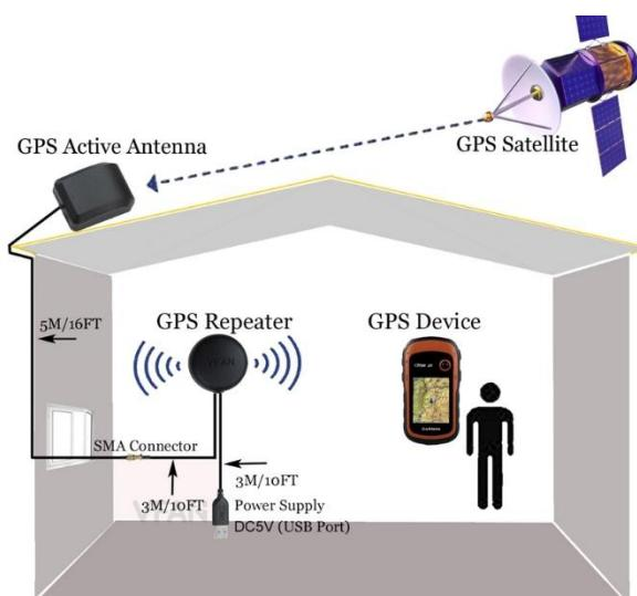
this GPS antenna with magnetic base, IPX5 waterproof. It usually consume 10 to 40 mA. Inside LNA along with antenna circuitry part.
