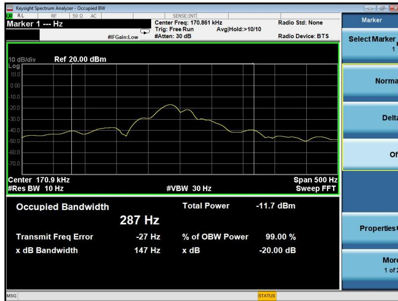
Note: The measured signal is Cw-like, adjusting the RBW per C63.10 would not be practical since measurement bandwidth will always follow the RBW. The RBW is set to 10 Hz to perform the occupied bandwidth test.
