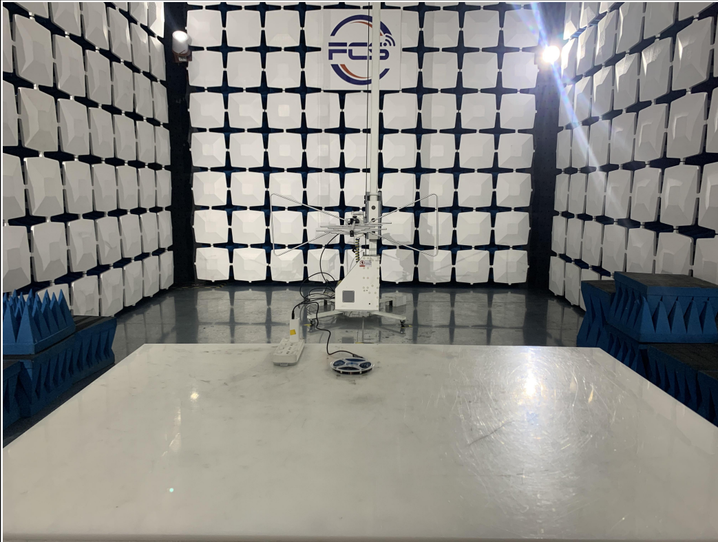
Above 1GHz for radiated emission test setup
