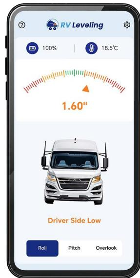
1.2. Each screen has a gauge, measurement number, vehicle image, and text guides at the bottom. These all work together to make the leveling process as easy as possible
