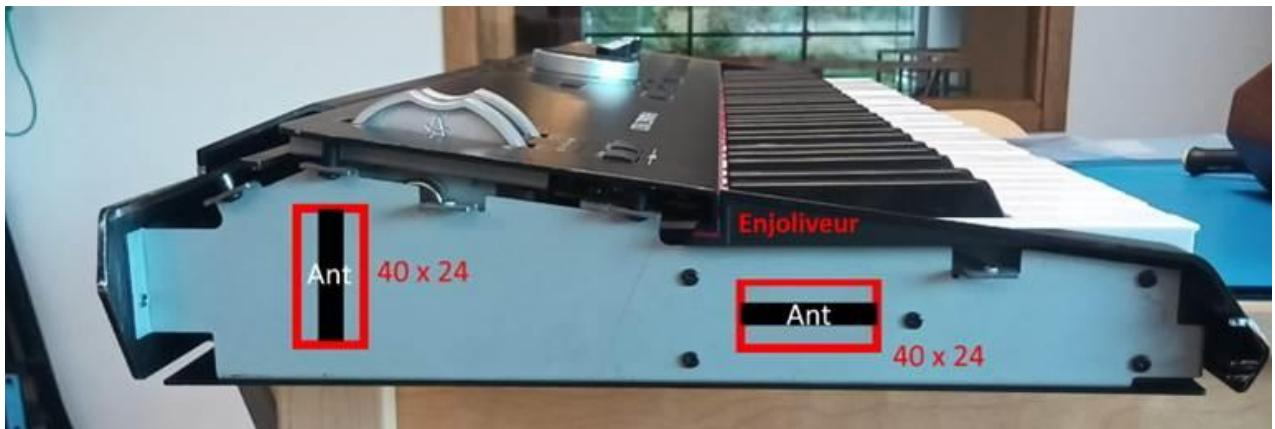
Important: To avoid losing too much rigidity and if necessary, the center of the window can keep a "rigidity bar" 2 to 3 mm wide, without impact on the antenna (only both ends of these dipole antennas work to develop the E-field):
