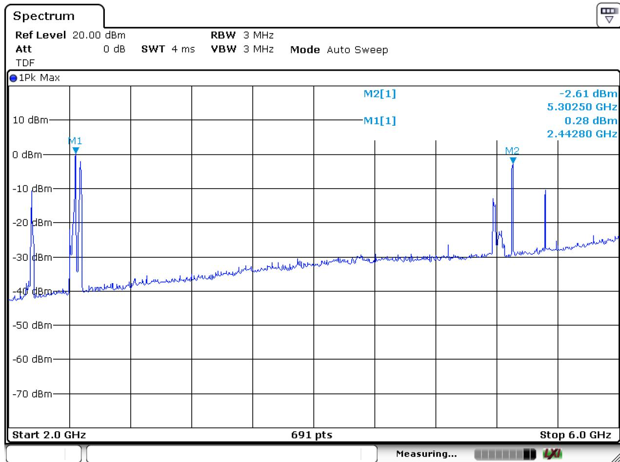
These gains are also good, and like the other antenna (although a little weaker, probably due to the aftertouch ribbon of the keyboard being a little too close). Same remark about the 5300 MHz necessarily a little disadvantaged.
