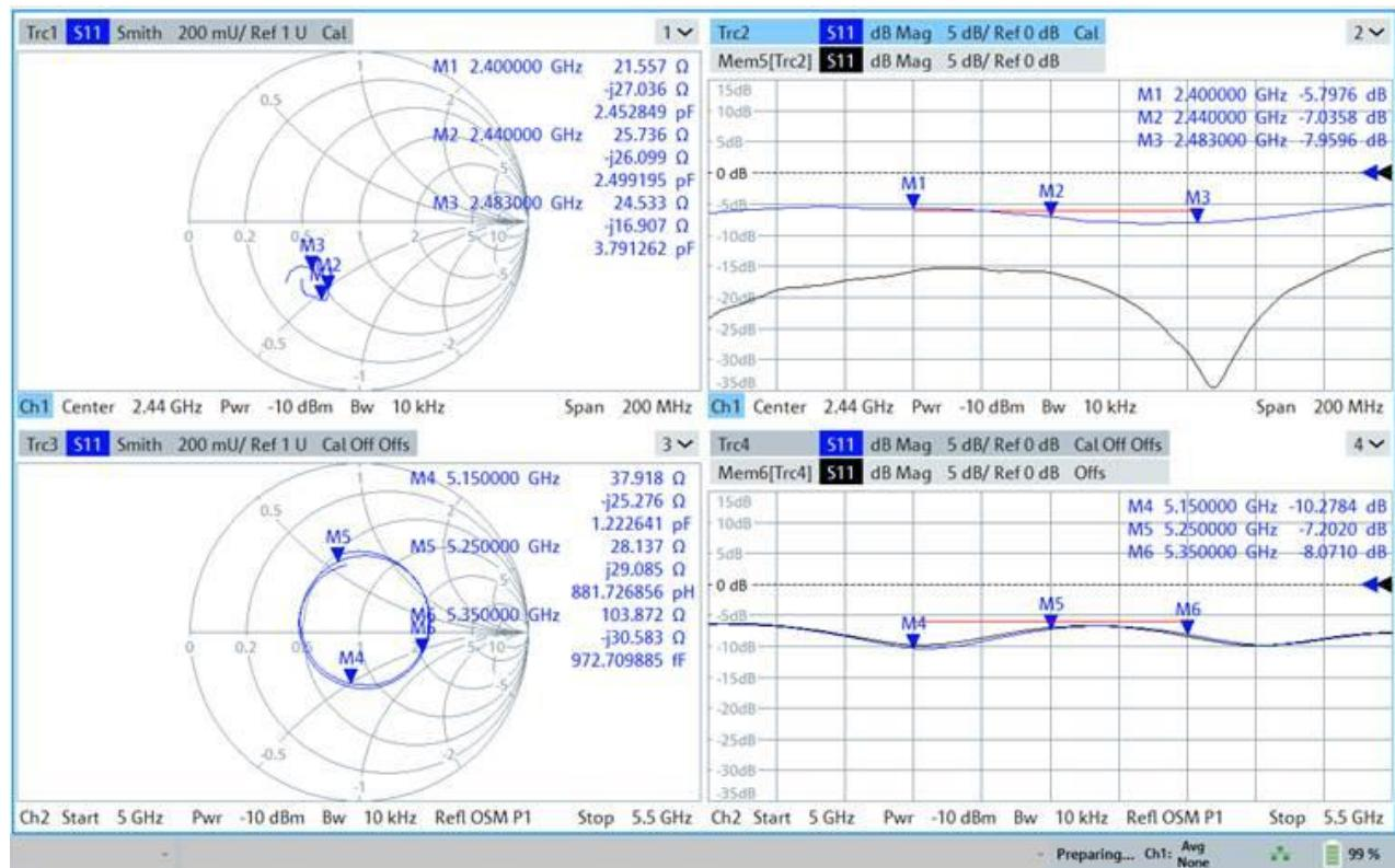
The M.Gear antenna can be placed 10 mm away from the metal, but the impact on the 5GHz becomes noticeable. It is therefore preferable to remove the metal immediately under the antenna.
