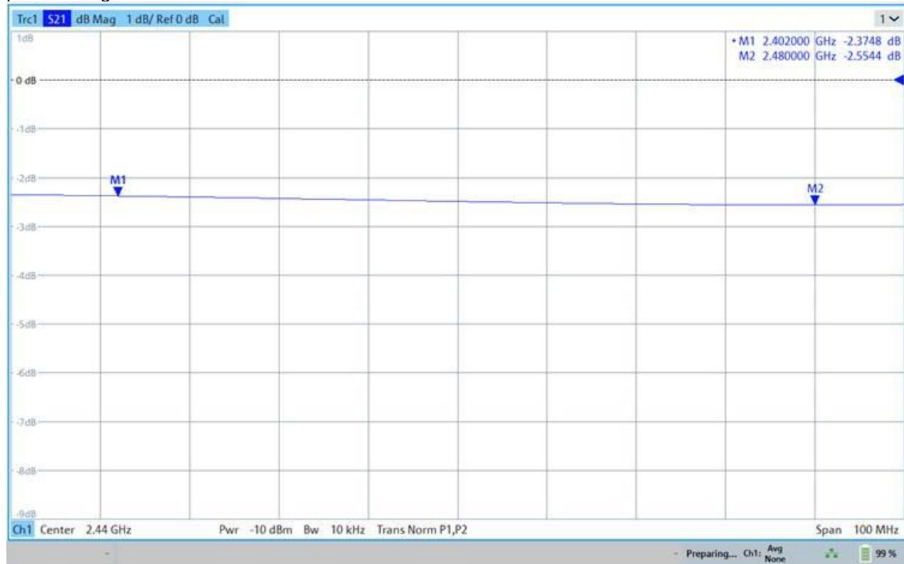
The average attenuation is 2.45 dB for 80 cm, i.e. 0.3 dB / 10 cm. A 1 m coaxial cable therefore "costs" -3 dB, i.e. a transmission power divided by 2, but an "indoor" range only reduced by 15 to 20%.
