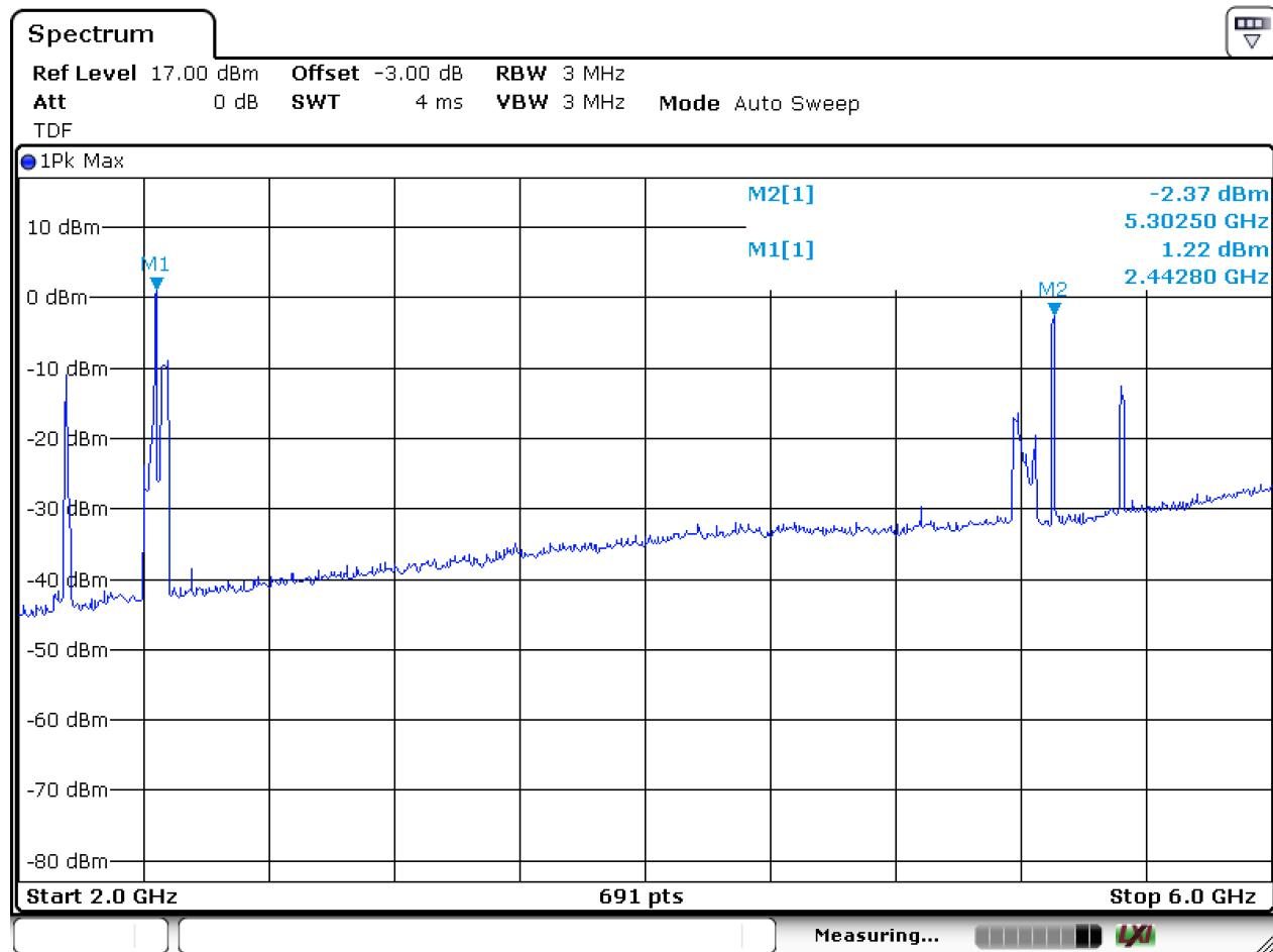
These gains are very good, given the integration. The 5300 MHz one is a little lower, as it is an additional element to this multiband antenna.
