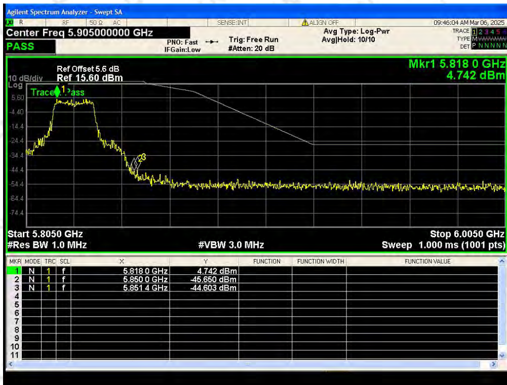
Band Edge NVNT 802.11ac20 5745MHz Ant1
