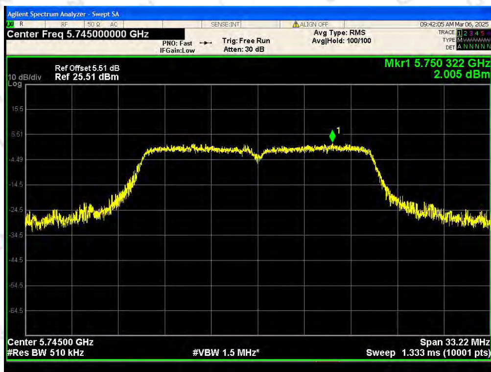
PSD NVNT 802.11a 5745MHz Ant1
