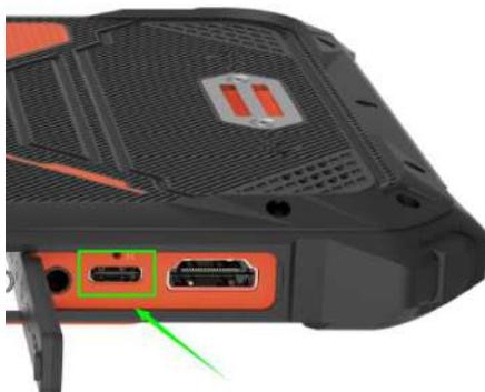
2. Connect the power adapter with Type-C cable to the USB Type-C port.
