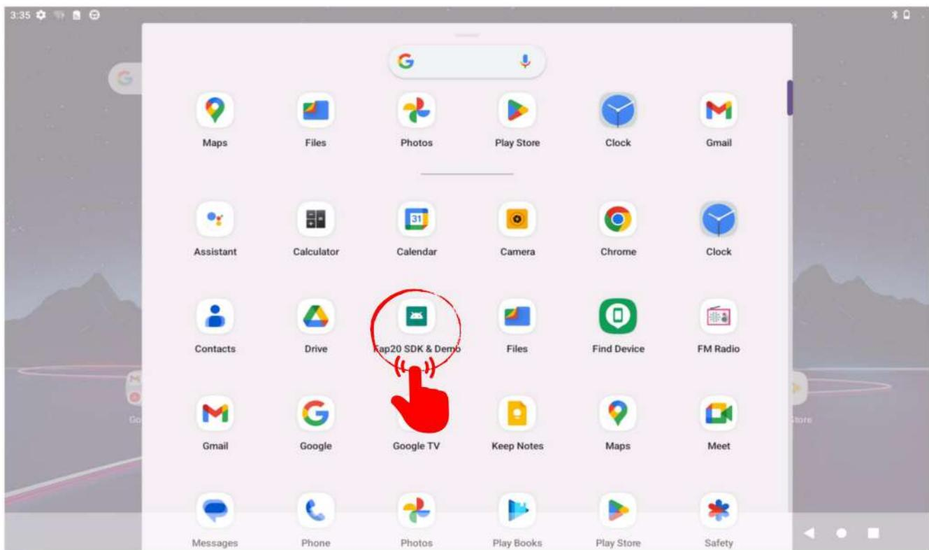
Select "Init", the fingerprint collection window at the lower right corner of the tablet will light up in red. Press your finger on it to complete the fingerprint collection.
