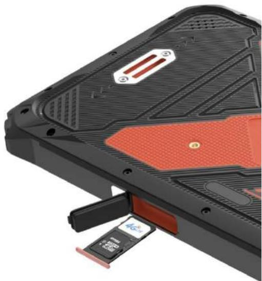
After installed SIM card slot, please close the I/O compartment cover.
