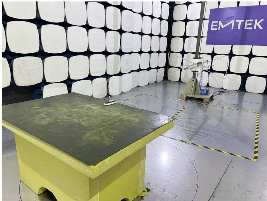
Spurious Emission Test Setup (Below 1GHz)
