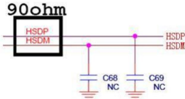
Note: USB D + / D-differential line impedance control 90 OHM; C 68 and C 69 should be reserved in advance and adjusted according to the actual situation;
