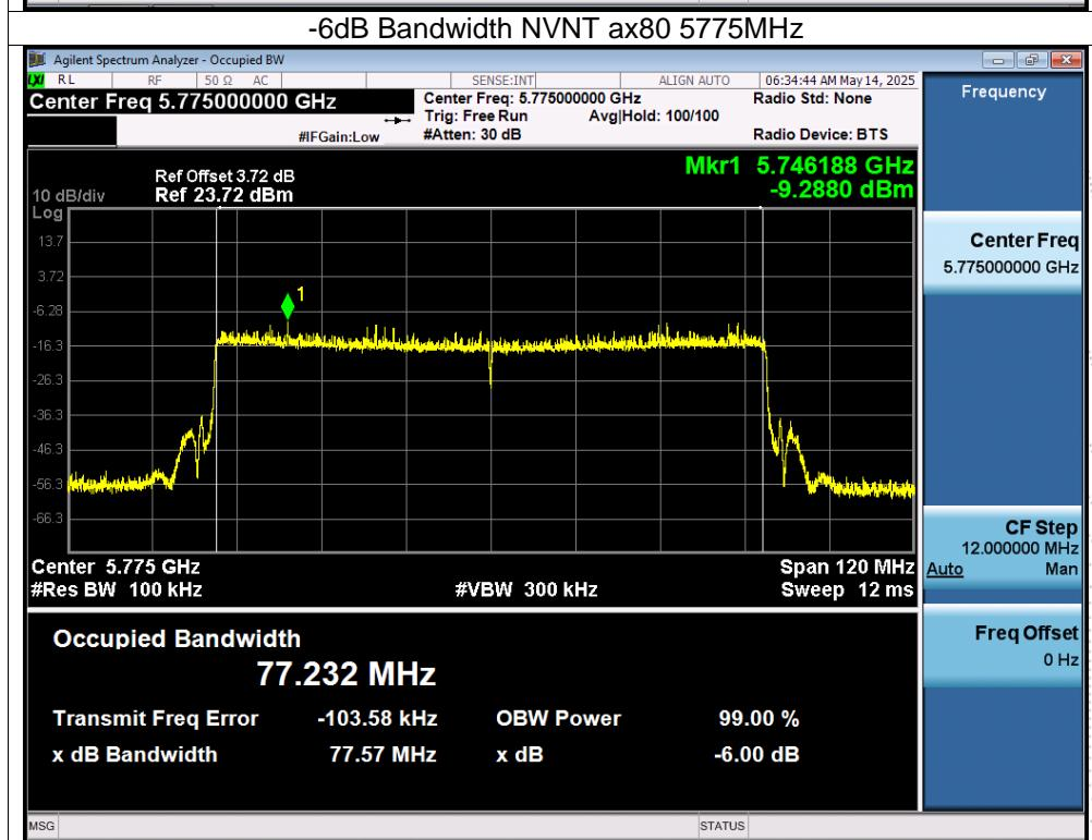
Note: A(B) Represent the value of antenna A and B, The worst data is Antenna A, only shown Antenna A Plot.
