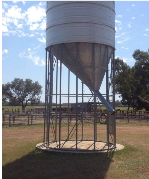
Figure 3: Example of silo with an asymmetric cone
