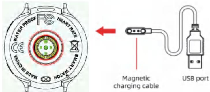
Place the magnetic charging wire near the charging port of the bottom shell, and it will automatically engage (pay attention to adjusting the direction). Insert the other end into a regular charging head until the charging indicator appears on the watch screen. This watch belongs to high-precision watches and has waterproof and dust-proof treatment. Please do not disassemble it yourself, and please pay attention to the following matters:
