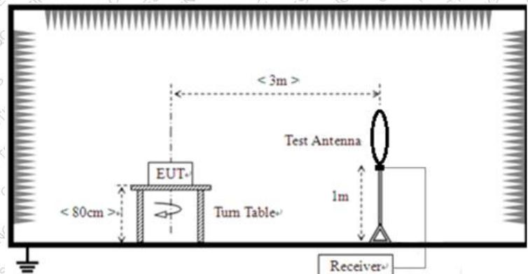
**For radiated emissions from 30MHz to 1GHz**
