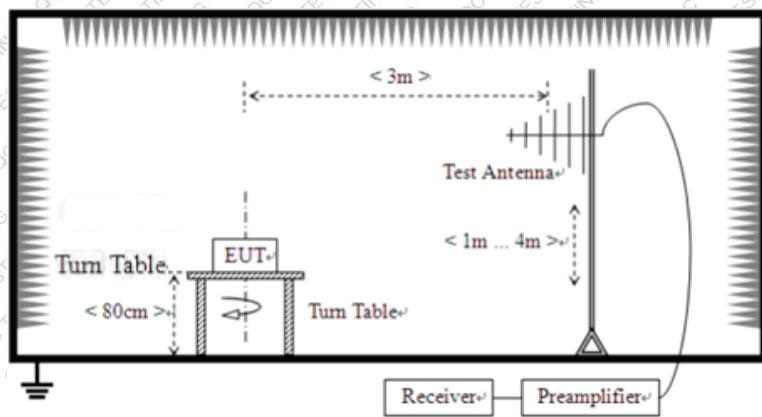
**For radiated emissions above 1GHz**
