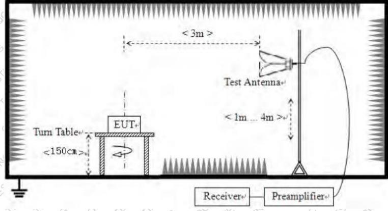
**8.2.4 EMI Test Receiver Setup**
