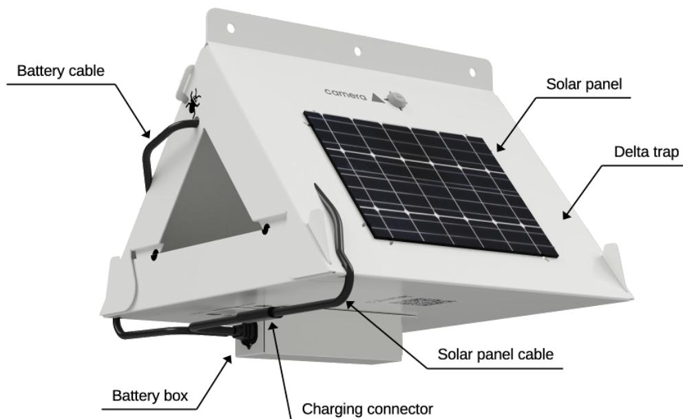
The battery should be connected to the scoutlabs Mini via the USB-C connector on the housing, while the solar panel should be connected to the charging connector (USB-C), coming out from the battery box. Operating the trap in normal mode is only recommended, when it is fully assembled, all of the connectors, cables and mounting points fixed.
