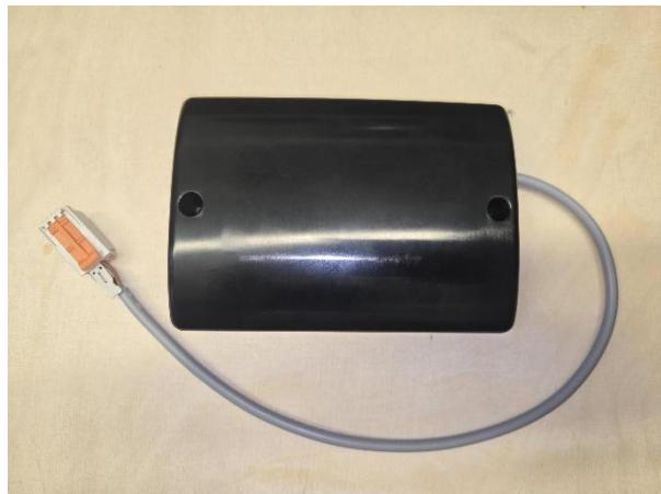
2. Add Wago connector on a  $3 \times 0.5 \text{mm}^2$  cable. Brown is 24VDC, Grey is an external pairing switch, Black is GND.
