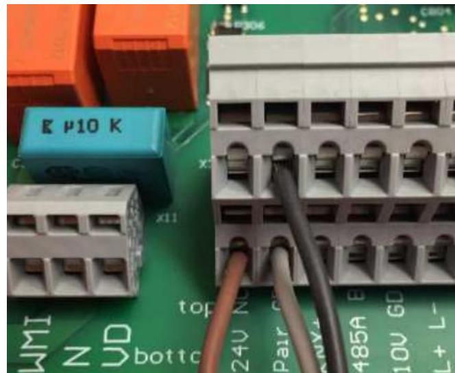
b. Connection on a power supply and a pairing switch connecting to GND (NPN).
