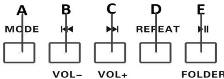
A. MODE: Short press: Press to switch between **USB / SD / BLUETOOTH** .
