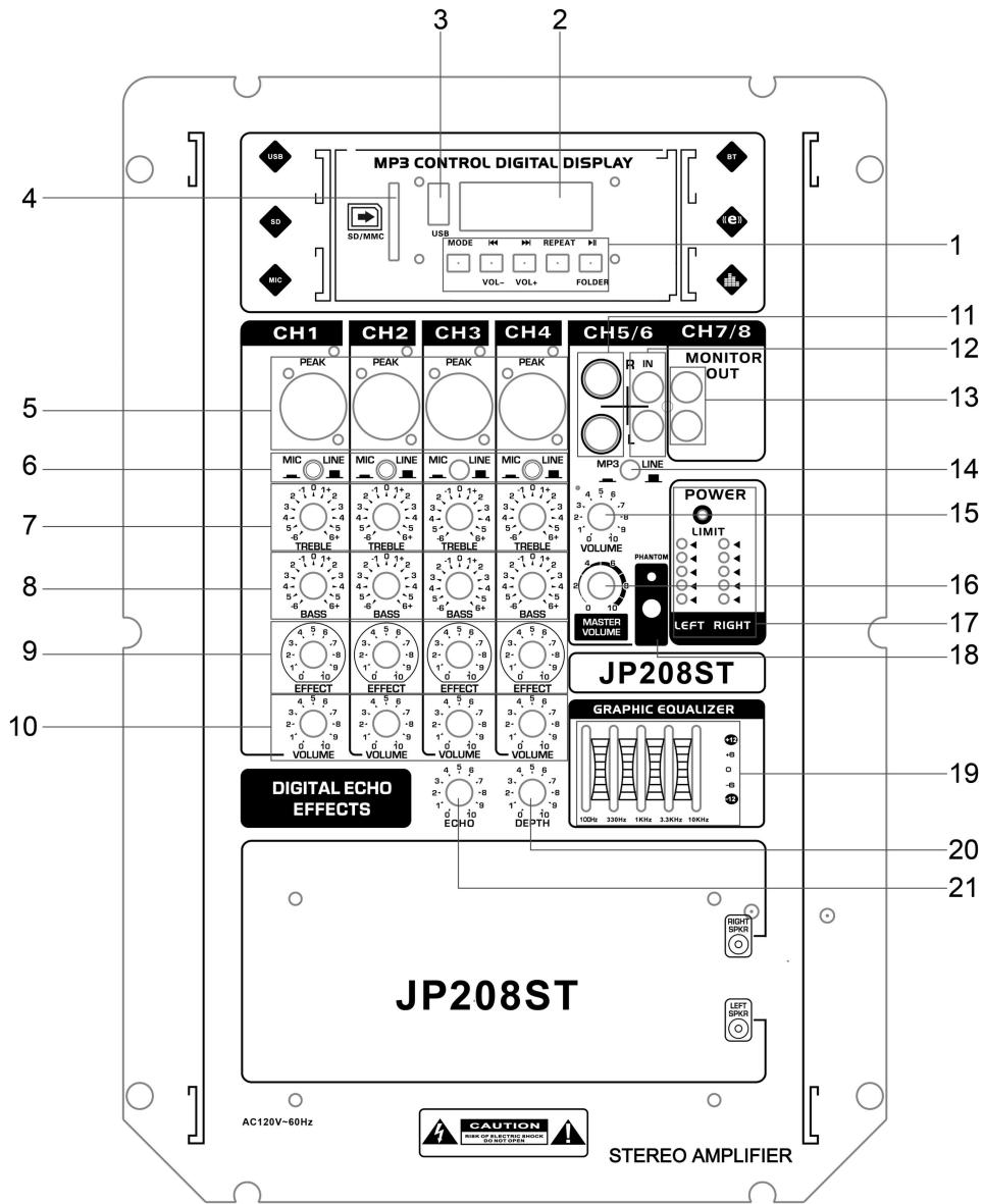
**5. Channel 1-4 XLR Connector:** Connect Microphone and Line input using the XLR cables.
