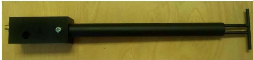
Figure 1 – MVG COMOSAR Validation Dipole
