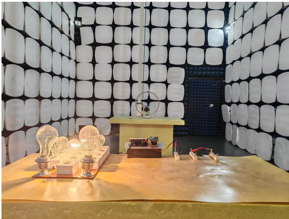
Radiated emission Test Setup (30MHz~1GHz)
