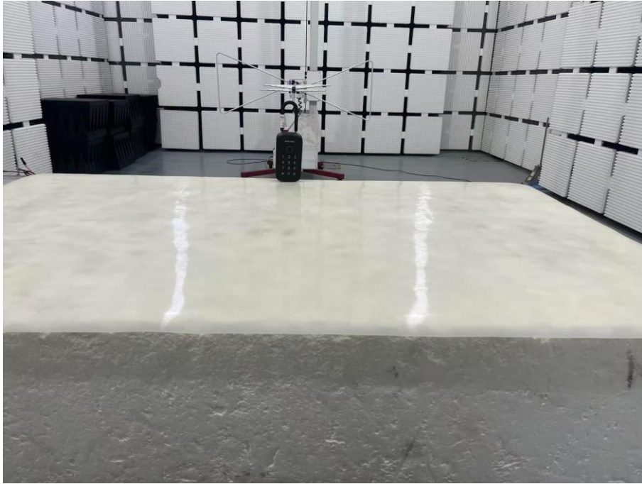
Set-up for Radiated Spurious Emission, Above 1GHz
