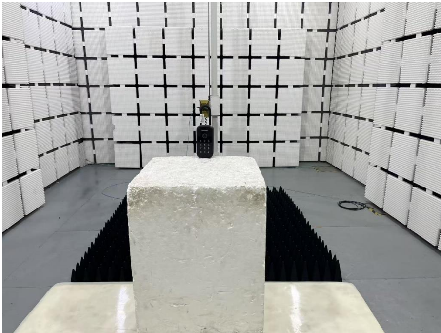
Set-up for Radiated Spurious Emission, Above 1GHz
