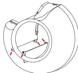
1. Disassembly & Assembly method of filter
