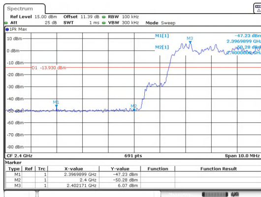
Out Of Band Emission(Left) 8DPSK_3-DH5_Channel Hopping
