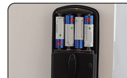
Step6 Install the batteries cover
