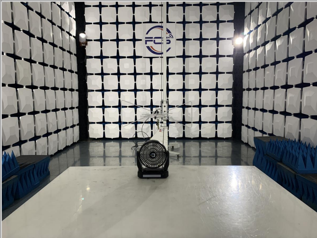
Above 1GHz for radiated emission test setup
