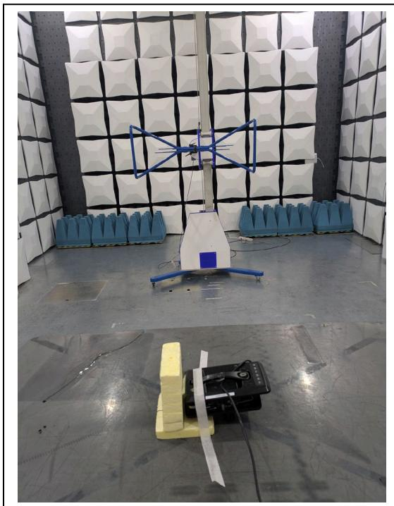
**Radiated Spurious Emission: 1 GHz to 18 GHz**
