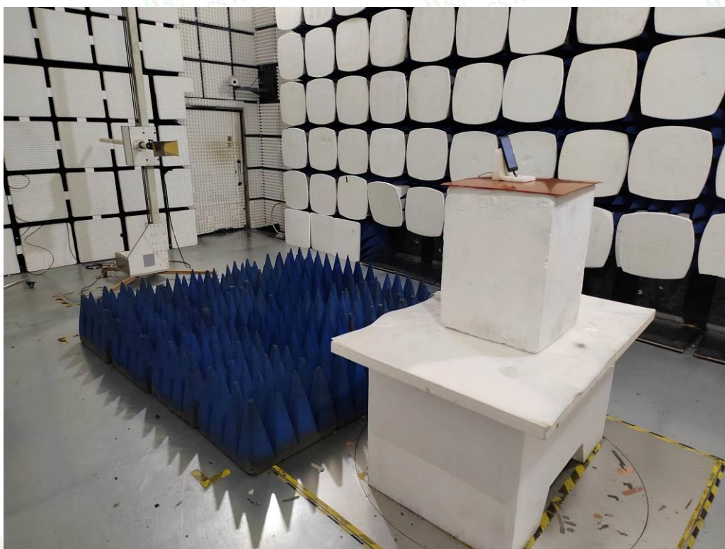
Radiated Emissions Measurement (Above 1GHz)
