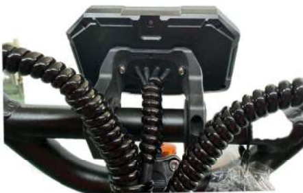
4. Check whether the brake handle, headlight switch, dual drive switch, and instrument are fixed
