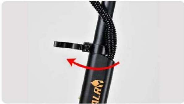
1. Open the fixing clips
