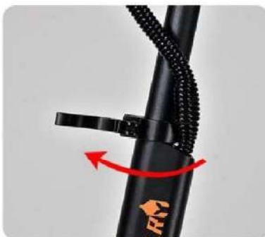
1. Open the fixing clips
