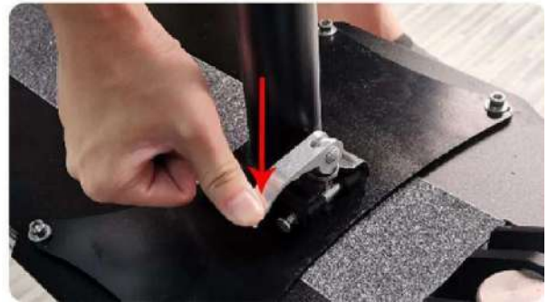
2. Tighten the fixed buckle
