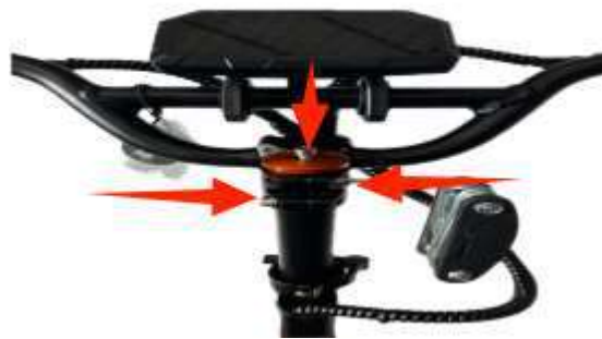
3. Adjust the angle and fasten it Screws
