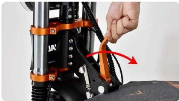
3. Release the stem lock switch
