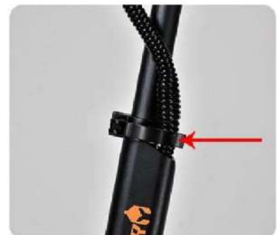
4. Snap-fit folding clips
