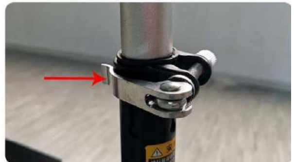
4. Tighten the fixed buckle
