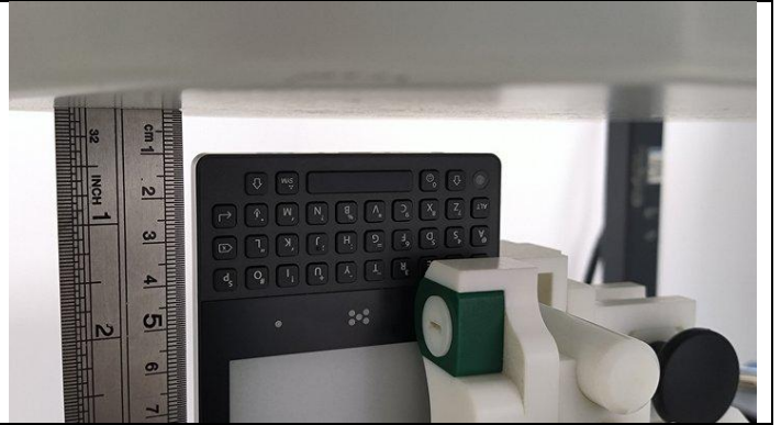
Bottom Side (Separation distance of 10mm)
