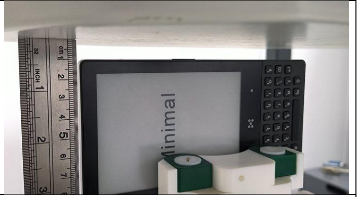
Bottom Side (Separation distance of 10mm)
