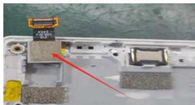
The bottom of the camera is grounded with a double-sided conductive cloth.
