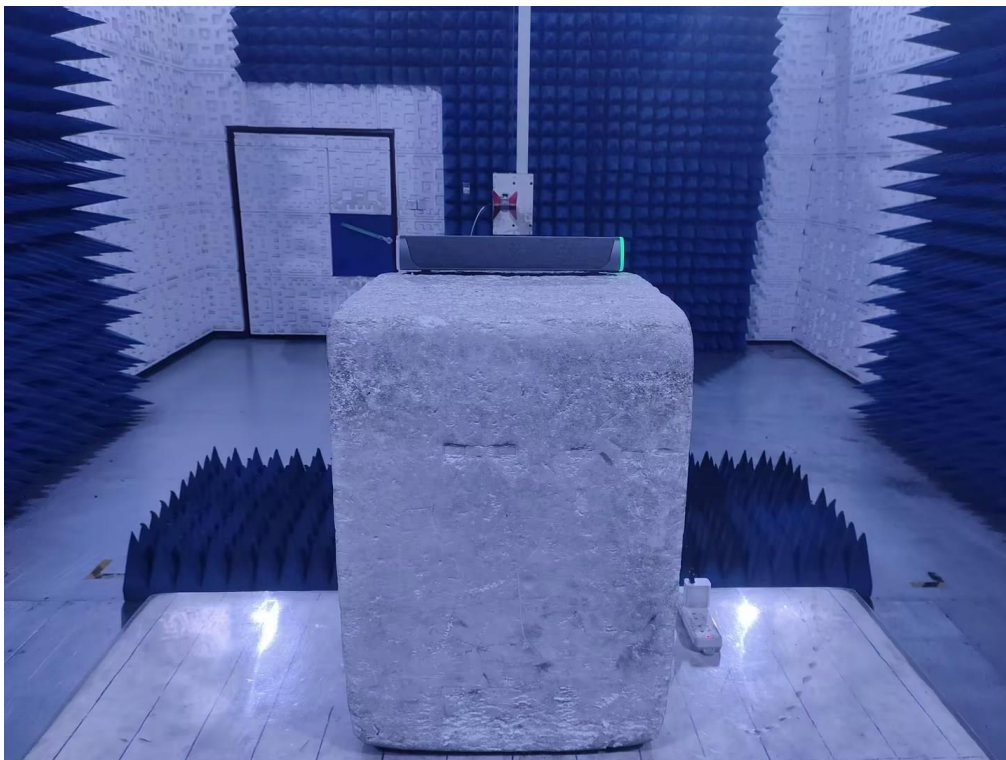
RADIATED EMISSION TEST SETUP ABOVE 1GHz
