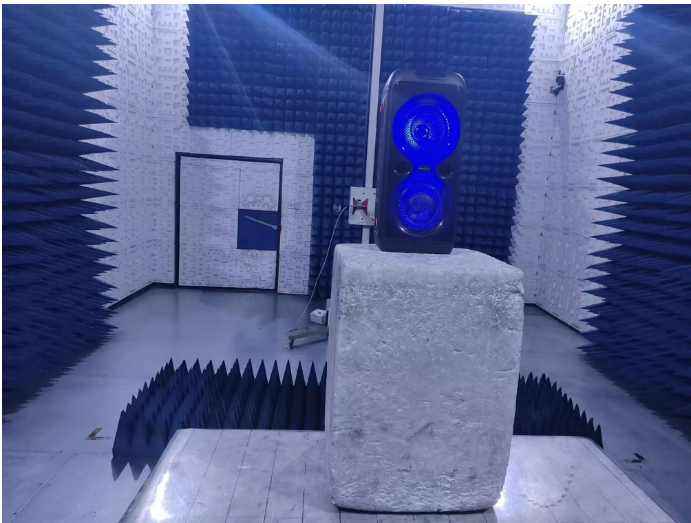
RADIATED EMISSION TEST SETUP ABOVE 1GHz
