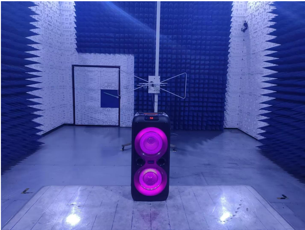
RADIATED EMISSION TEST SETUP ABOVE 1GHz
