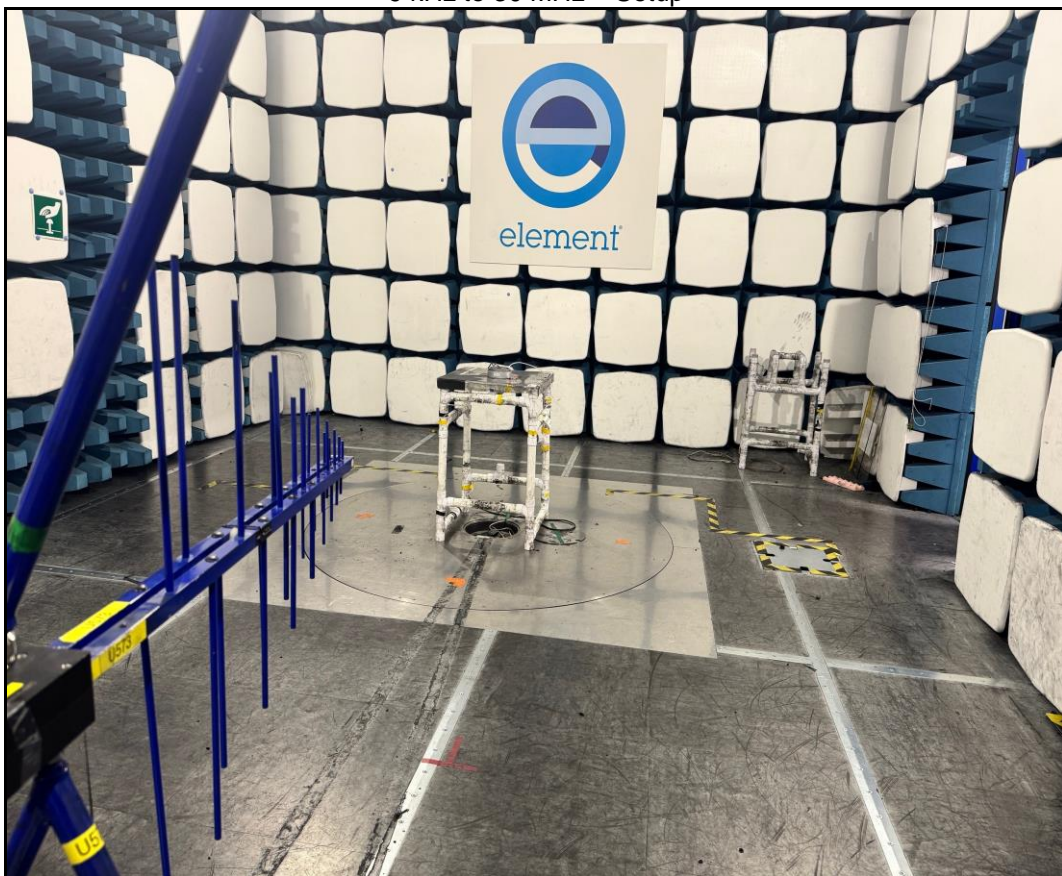
30 MHz to 1 GHz – Setup
