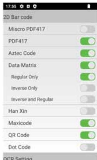
In The "Decode setting", you can configure settings for most of the commonly used ID and 2D codes.
